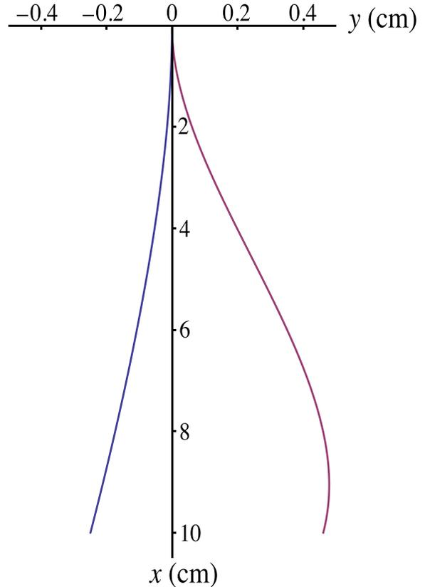
Fig. 4. Spring shape for the low-frequency resonance ( $\Omega = 60$  rad/s) on the left and the high-frequency resonance ( $\Omega' = 3800$  rad/s) on the right. The calculation is carried out using  $\chi = 2.1$ ,  $l = 10$  cm,  $h = 10$  cm, and  $\rho = 5$  cm.
