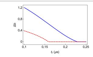
**Figure 5.** Difference between ideal and actual value of b at the end of the rotation versus final time for the optimized inverse-engineered protocol for rotations without (solid blue line) and with final squeezing ( $\gamma^2=3$ , dashed red line). The trap frequency is  $\omega_0/(2\pi)=2$  MHz, and the final rotation angle  $\theta_{\rm f}=\frac{\pi}{2}$ .
