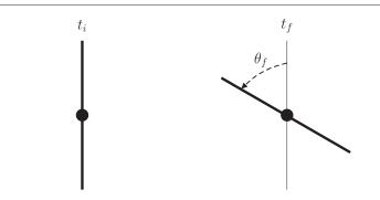
**Figure 1.** Schematic representation of the rotation process. The ion is confined along a line (where it is subjected to an effective one-dimensional-longitudinal-potential), which is rotated by an angle  $\theta$  up to  $\theta_f$  in a time  $t_6$  so that the final state is not excited.
