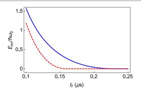
**Figure 4.** Final excitation energy versus final time for the optimized protocol without (solid blue line) and with final squeezing ( $\gamma^2 = 3$ , dashed red line). The trap frequency is  $\omega_0/(2\pi) = 2$  MHz, and the final rotation angle  $\theta_{\rm f} = \frac{\pi}{2}$ . The initial state is the ground state of the trap.
